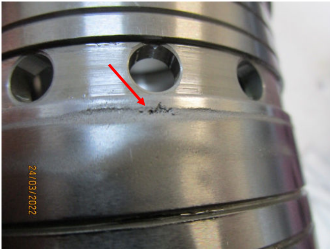
Ph. 7 - Distributor - Replace, deep cavitation.
