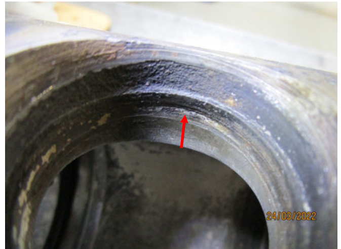
Ph. 2 - Seal Housing - Weld and rebores Oring seat.
