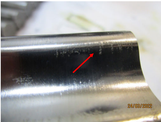
Ph. 9 - Rotation Motor - Wear evident, acceptable for re-use.
