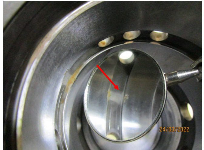
Ph. 8 - Rear Cylinder - Polish, light cavitation.
