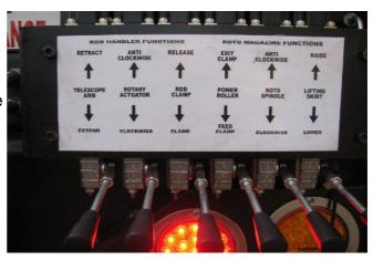
These functions are also controllable via radio remote wireless pendant!
