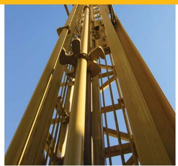
To assure long life, all mast structures are designed with double-cut lacing in high stress areas. There are several application-specific masts to choose from.
