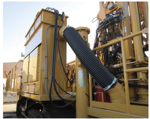
For efficient dust collection MD6240 has a dust collector rated at 127 m³/min (4,500 ft³/min) and separate water injection system. Both dry and water injection systems can be mounted on the same drill.
