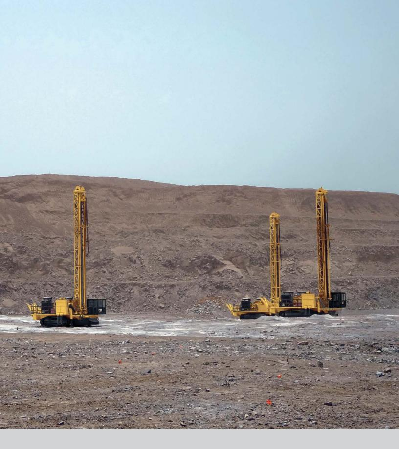
High productivity and low cost of ownership is yours with the MD6240 Rotary Drill. With bit load force of 24 000 kg (52,911 lb) and the capability to drill depths up to 55.47 m (182 ft) the MD6240 is well equipped to drill in hard or soft rock applications. Built to be reliable, safe and easy to service for years to come.
