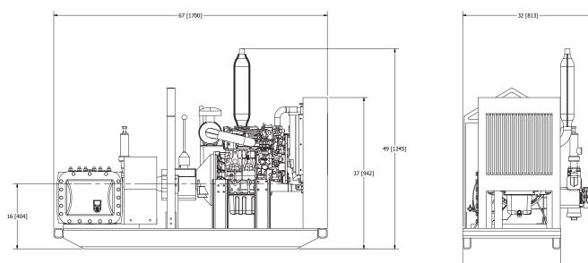
dimension in inches (mm) 564 kg/1185 lb (with oil, without battery)
